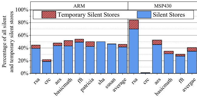
Figure 3. Percentage of (temporary) silent stores in Mibench 2 on MSP430 and ARM Cortex M* architectures, obtained with the ORACLE. On average, 40% (5%) of the total number of store instructions are (temporary) silent.
